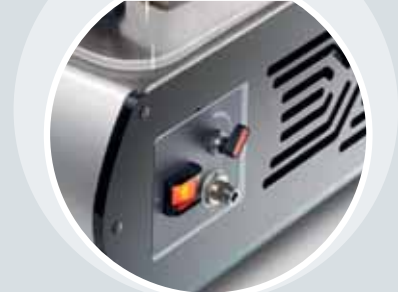
14 - Optional gas inerte e soft air Inert gas system and soft air option
